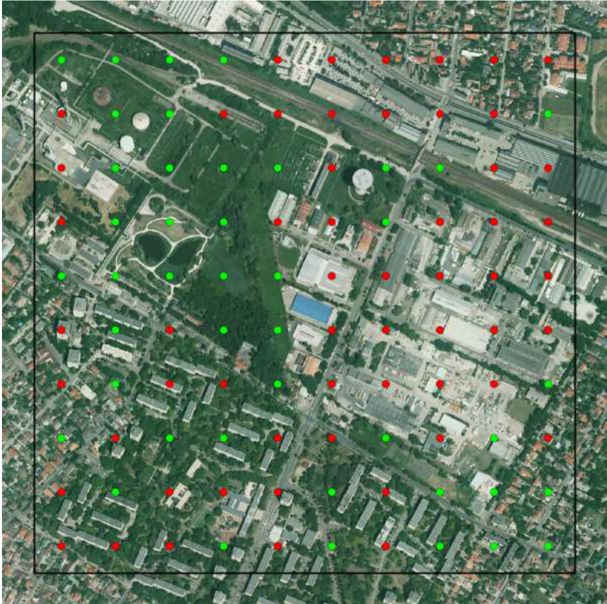
Figure 5.1.a: Reference interpretation of sealing within a 1x1km PSU for year 2018 (green: non-sealed, red: sealed).
