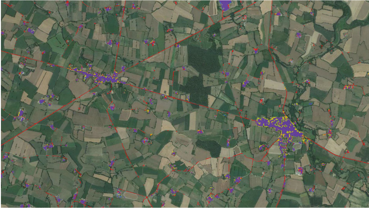
Figure 4.1.1.c: More detailed appearance of secondary road network in CLC+ Backbone 2018. Red: CLC+ Backbone 2018; Blue: IMD2018 \geq 30%; Yellow: IMD2018: 1-30% Purple: CLC+ Backbone 2018 & IMD2018 \geq 30%; Orange: CLC+ Backbone 2018 & IMD2018: 1-30% France, x,y= 3500754,2818803 (EPSG:3035)
